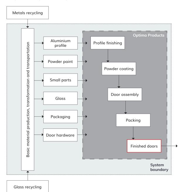
SYSTEM BOUNDARIES (A1-A3) FOR MANUFACTURING FACILITY-PRODUCED GLAZED DOOR LCA
