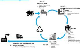
The diagram illustrates the life cycle stages of construction products in general. The system boundaries starts with the raw materials for the production of the three layers of the Urbanscape® System. These are manufactured separately before being assembled.
