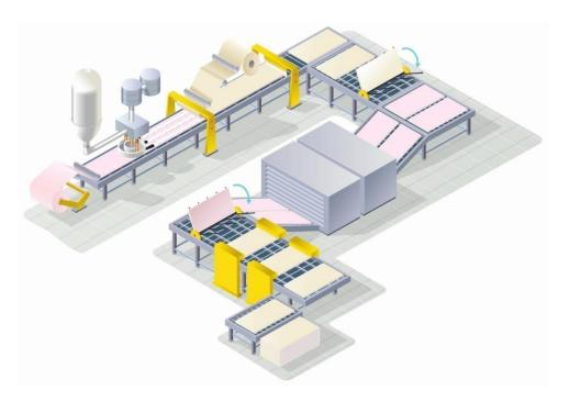
Raw materials are homogeneously mixed to form a gypsum slurry that is spread via hose outlets onto a paper liner on a moving belt conveyor. As second paper line is fed onto the production line from above to form the plasterboard. The plasterboard continues along the production line where it is finished, dried and cut to size.
