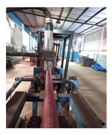
After produce the bare pipes if required by customer, by using of water based paint, Pipes may be protect. It is used in application areas such as firefighting and utility water to increase corrosion resistance.
