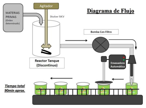
Figure 3. Graphene lime production process.
