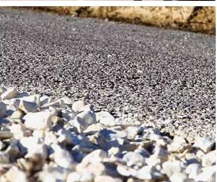
Tests carried out according to the Standard EN 206 establishes the compressive strength of i.idro DRAIN at a minimum of 10 MPa. The use of i.idro DRAIN does not require particular performance as regards environmental exposure class and workability. There is therefore no defined exposure class nor slump class.
