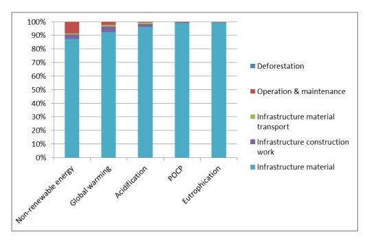
Emission impact categories and the relative contributions (in %) made by the process groups relevant to the Bothnia Line's power, signalling and telecom systems. The process groups include all activities during the lifetime of the infrastructure. For example, "Infrastructure material" covers all materials used during construction, maintenance and reinvestment.
