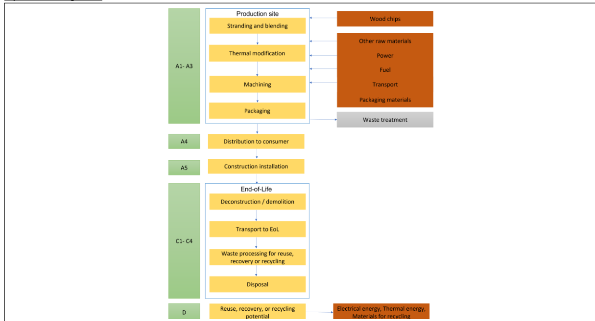
Figure 2: Process flow diagram showing the production and distribution of Norbord MDF
