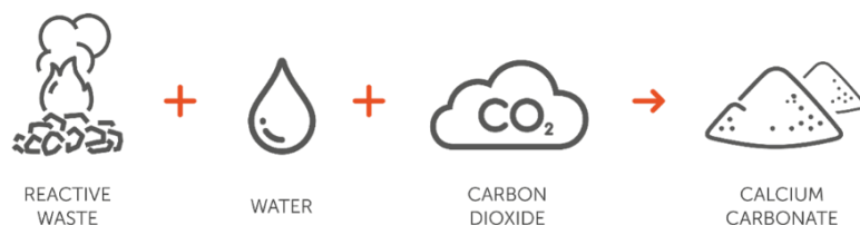
Figure 1: Basic accelerated carbonation reaction
