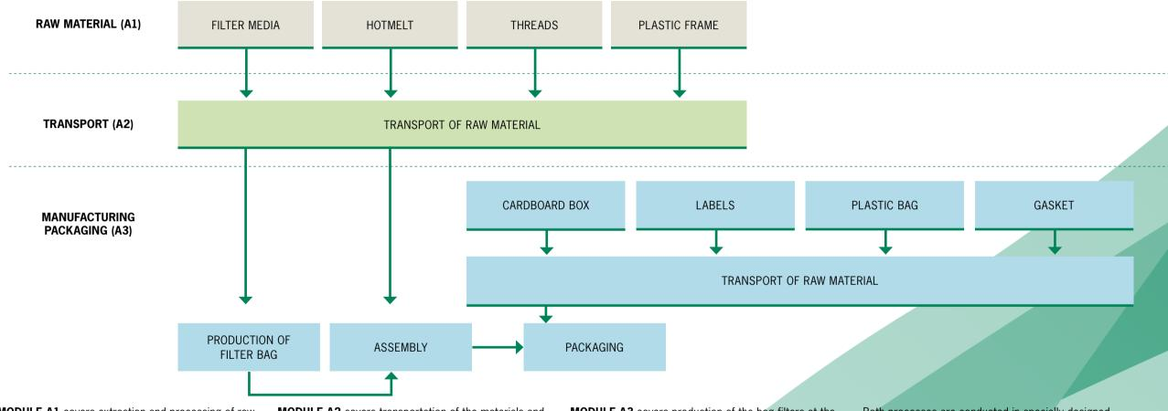
**MODULE A1** covers extraction and processing of raw materials, as well as production of the materials and components used for production of bag filters: filter media, plastic frame, hotmelt and threads.
