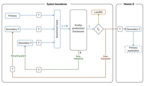
R – Process losses T<sub>R</sub> – Recovery Rate Y – Smelting yield T - Transport
