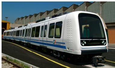
MLA Metrobus Brescia consists of three car bodies with two articulations. The traction is supplied by six electric engines, coupled on three of the four bogies; the fourth truck is a trailer one.
