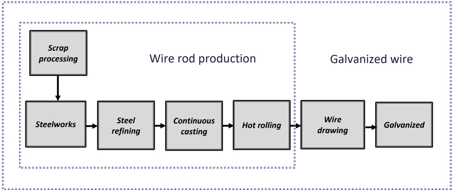
Figure 1. Flow diagram of wire rod and galvanized wire manufacturing process
