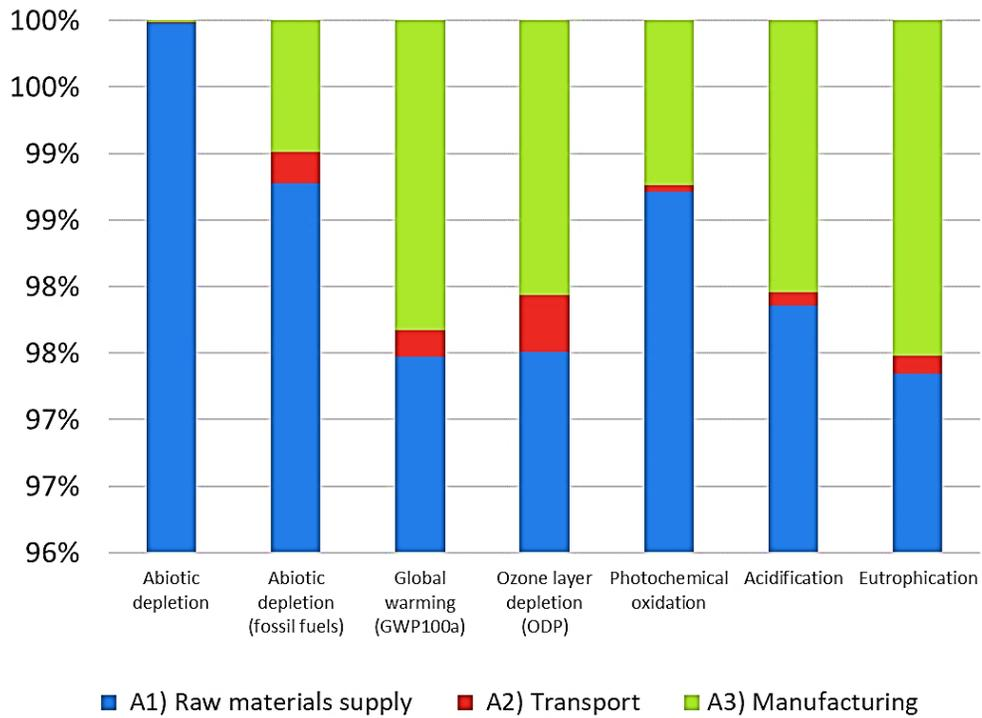
Figure 3. Potential environmental impact contribution per metric ton of galvanized wire
