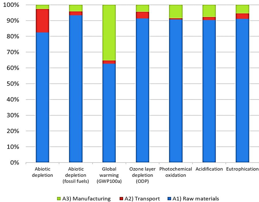
Figure 2. Potential environmental impact contribution per metric ton of wire rod
