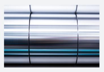
Aluminium foil is produced by rolling aluminium slabs cast from molten aluminium in a rolling mill to the desired thickness. To maintain a constant thickness, a technician monitors the rolling mill sensors to ensure the pressure on the slab is correct. It is then coiled and sent to the cold rolling mill. To avoid breakage because of the thinness, the foil is doubled in the cold rolling mill and the rolled to the desired thickness.
