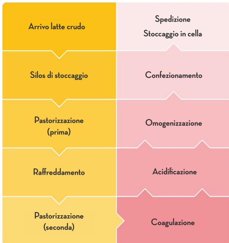
FIGURA 2 – IL PROCESSO DI PRODUZIONE DEL MASCARPONE.
