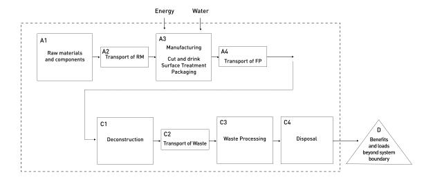
Flowchart with system boundaries. Modules A1-C4 are within system boundary (dashed line). Module D is outside system boundary but is also modeled.
