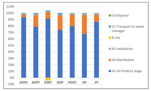
Figure 5. Potential environmental impacts of the life cycle of  $1m^2$  of Graphenstone<sup>®</sup> NaturMortar Base.
