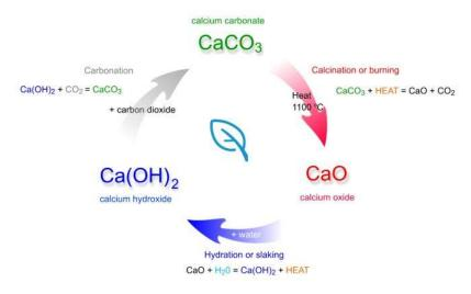
Figure 4. Lime cycle: Calcium carbonate-Calcium oxide-Calcium hydroxide.
