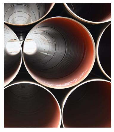
The main application field of solvent-free epoxy paint is fresh water lines. This kind of process cures a coating with excellent corrosion resistance to fresh water, sea water, crude oil and abrasion. It is applicable in thick coats by standard heavy duty airless spray equipment. Harmless to grain cargo. It uses as a lining in potable water tanks and pipelines, where solvent-free materials are required.
