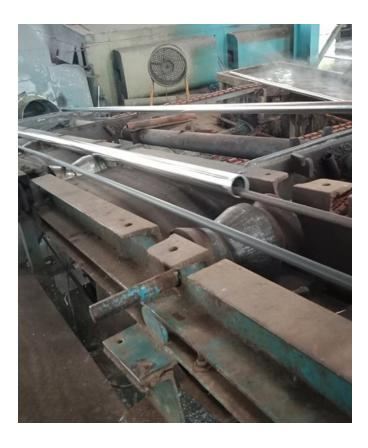
After produce the pipes if required by customer, by using of zinc pipes may be coated by hit dipped galvanizing. It's used in many application areas such as supply of liquid, Gases and makes the greenhouses & other fabrication job, pipes to protect them against corrosion and to extend their service life.
