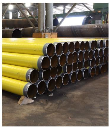
A dust coating is sprayed onto the cleaned and warmed pipe, creating a sticky coating. When the pipe is hot, liquid polyethylene band is wrapped around the pipe. In order to protect the outer surface against corrosion and to prolong its lifespan, three layers of polyethylene or polypropylene coating are applied. The coating is in accordance with DIN 30670, 30678, TS 5139 and UNI 9099 standards.
