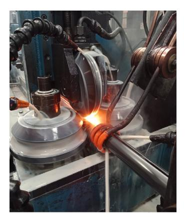
Bare Steel Pipes are manufactured longitudinally welded with source of high frequency (ERW) from the strips having steel grade at their manufacturing standards. Our standard productions are packaged hexagonally with steel strips. According to customer demands, product may be packed with HDPE clothe as well.
